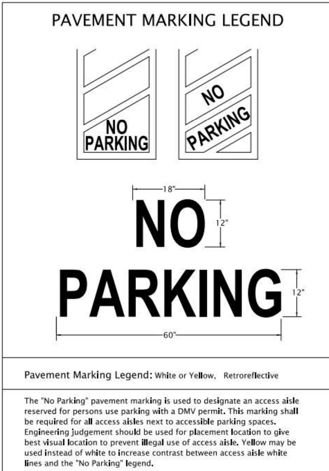
Figure 7: Pavement Marking Legend details for NO PARKING
